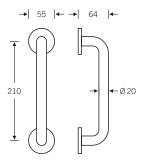
Double-action swing doors in restaurants, canteens, hospitals and so forth are generally fitted with both push and pull plates for added protection. An alternative arrangement is conceivable in the gripping area, however. Furnishing the two faces of the door with the combination shown above allows the desired direction of swing to be implied.
