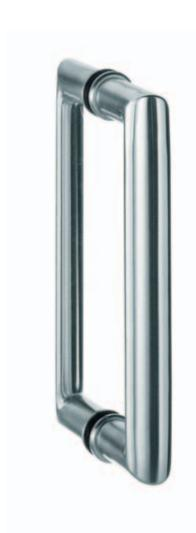
FSB could not resist squeezing all the experience gained in fashioning the  $40 \times 28$  mm oval tube into a smaller diameter. And thus it was that the standard in-line pull FSB 6650 came into being .lt features a skewed oval grip 36 by 22 mm in diameter affixed to circular supports.
